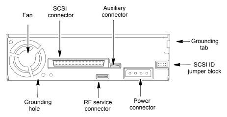
Figure 1-4 Internal tape drive: back-panel components
